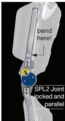
DO NOT compensate for flexion by unlocking the SPL2 joint.
