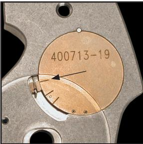
Position of Lever Arm when Satellite Slide Lever is in Manual Unlock Position
