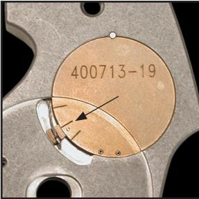
Position of Lever Arm when Satellite Slide Lever is in Automatic Lock Position
