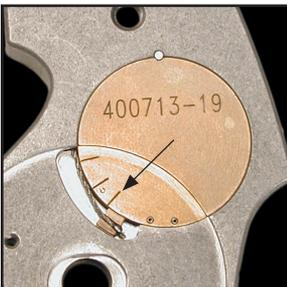
Position of Lever Arm when Satellite Slide Lever is in Manual Lock Position
